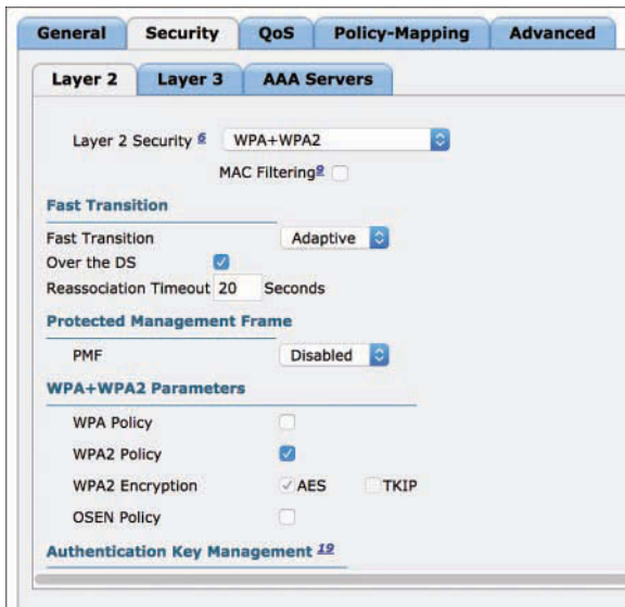
Figure 11-27 Layer 2 Security Subtab for ISE Corporate WLAN
