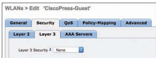
Figure 17-8 Layer 3 Security Subtab Configuration for CiscoPress-Guest
