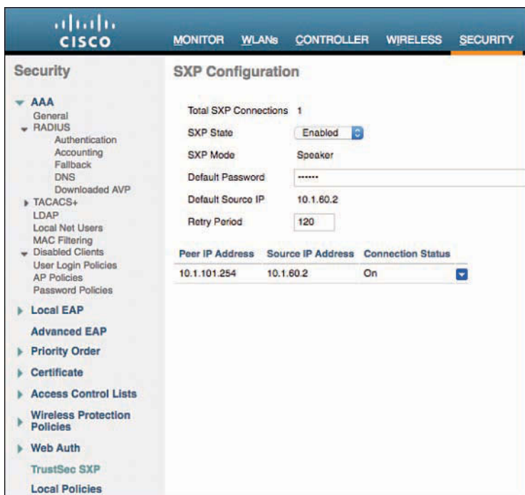
Figure 22-14 SXP Connection on WLC
