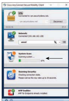
Figure 19-44 AnyConnect System Scan Module in Progress
