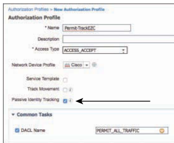
Figure 23-38 Authorization Profile with Passive Identity Tracking Enabled
