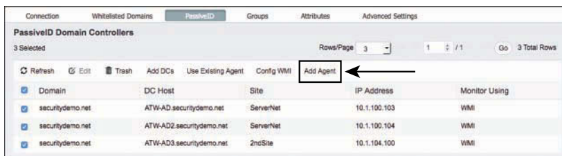
Figure 23-14 PassiveID Tab, Servers Selected to Be Monitored
