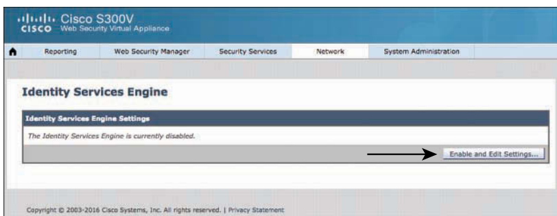
Figure 24-23 Editing the Identity Services Engine Configuration on the WSA
